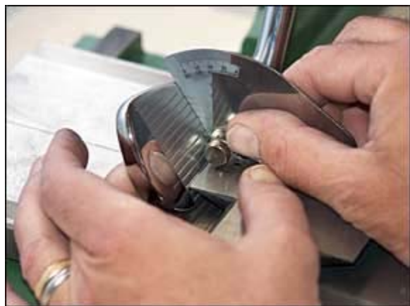
(photo 4) When using a hand held protractor, you must keep the face square while taking the measurement for loft.
