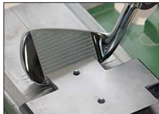
(photo 3) There is no "if, and or but" about using a device to square the face of an iron or wedge head for accurate loft measurement. It is impossible to measure the loft without one.
