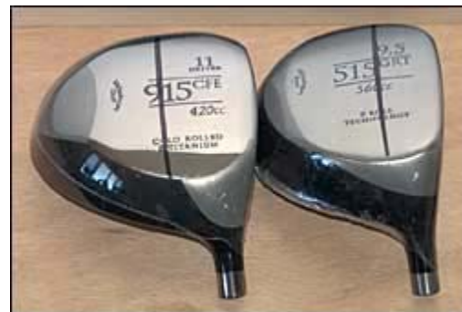
(photo 6) Here you see an example of how the face-to-back point of contact on the specs-measuring machine can be different for different woodhead designs. Again, this is because of the effect of the head's CG and size on how the head sits naturally in its address position.
