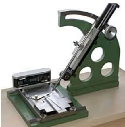
(photo 1a) While I use a very heavy duty specs-measuring machine, there are a number of equally accurate, quality made and affordable clubhead measuring machines that are available to clubmakers.
