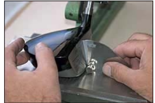
(photo 7) GENTLY hold the head in position with one hand while the other positions the loft protractor against the proper position on the face for loft measurement
