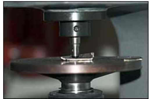
New QC toy #1 – Rockwell Hardness machine testing a section of the 515GRT 3-wood face to monitor the correct heat treatment of the T275 steel used to manufacture high COR fairway woods
