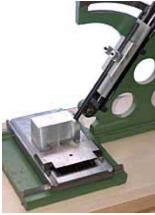
(photo 1b) Photo of the "Green Machine" with a specially made block perfectly machined to a 55 degree lie, 10 degree loft and 0 degree face angle that I use to periodically check the accuracy of my specs-measuring machine.
